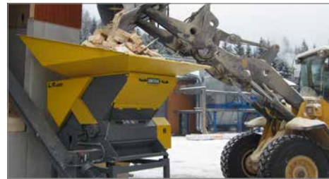
Application: Sawmill waste Solution: LR1400 Options: Additional hopper, screw conveyor Location: Austria
