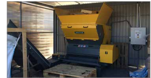
Application: Pallets Solution: LR1400 Options: Additional hopper, conveyor for metal deposition Location: Croatia
