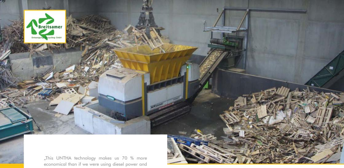
economical than if we were using diesel power and 30 % more economical than the conventional stardelta drive. The low speed nature of this shredding system also keeps the noise of our pellet production at a very low level, as well as producing a very low amount of fine particles."
